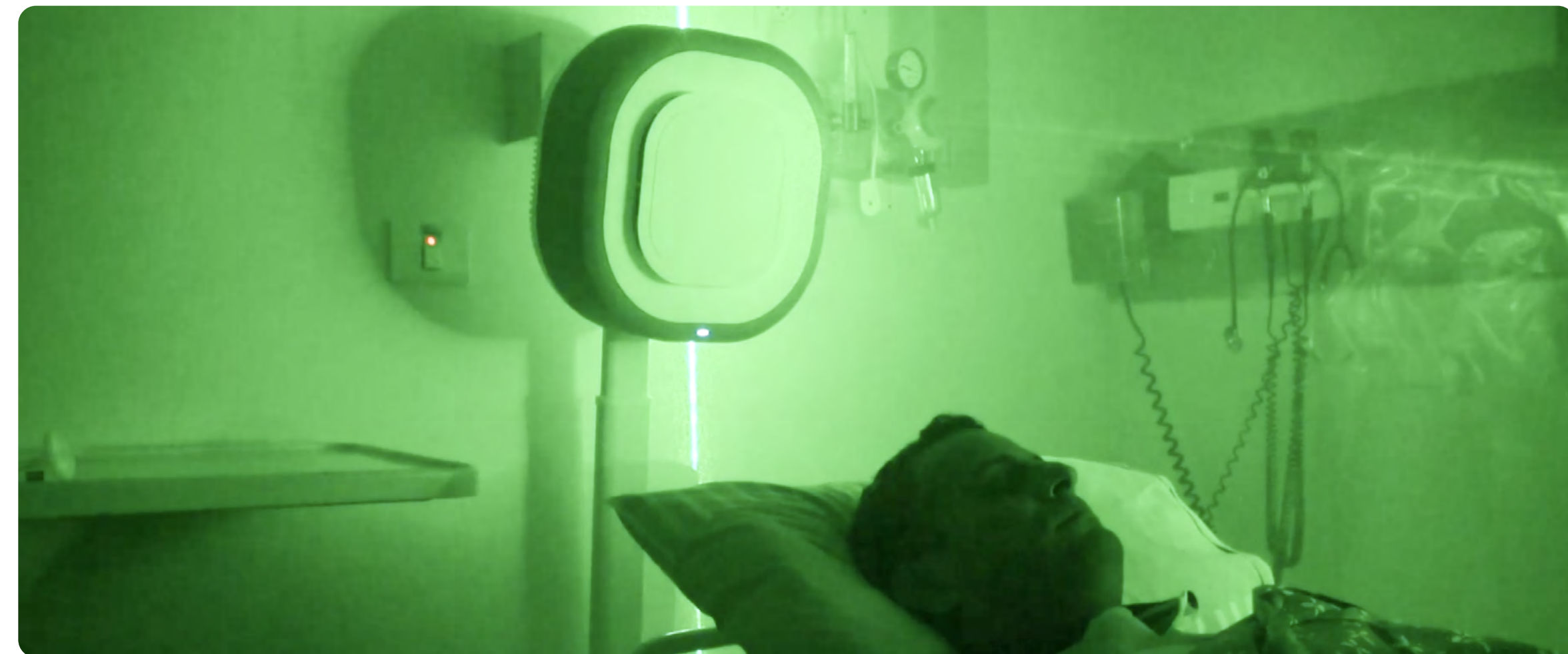
Using a laser light, smoke particles were illuminated in the room environment
